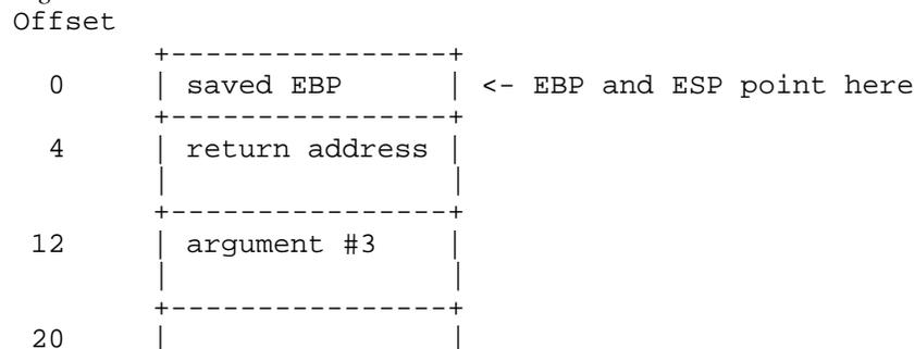
As the above diagrams show, the third argument is at offset 8 from register EBP in a small code model and offset 12 in a big code model.
