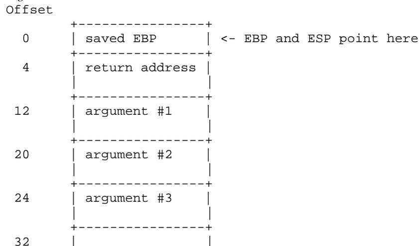
As the above diagrams show, the arguments are all on the stack and are referenced by specifying an offset from register EBP.
