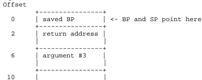
As the above diagrams show, the third argument is at offset 4 from register BP in a small code model and offset 6 in a big code model.
